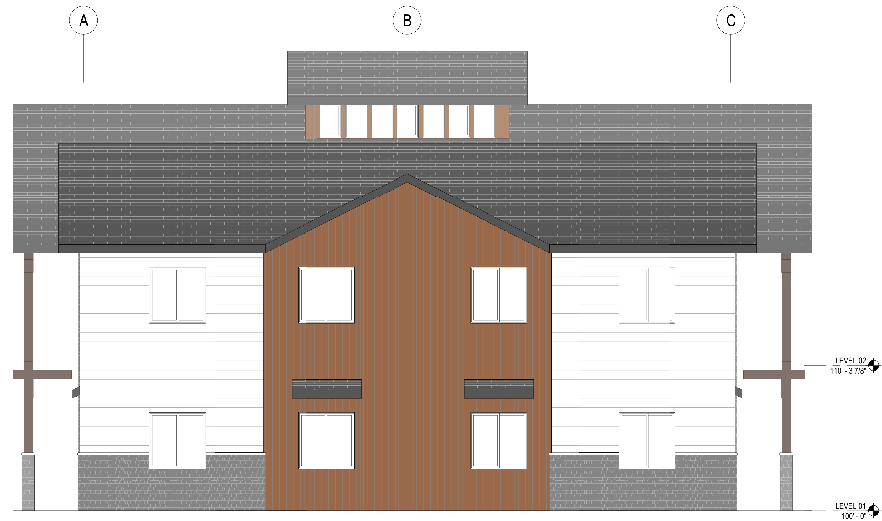
C4 EXTERIOR ELEVATION - OUTSIDE 1/4" = 1'-0"
